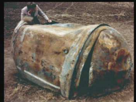
▲ LONE STAR The main propellant tank of the second stage of a Delta 2 launch vehicle landed near Georgetown, Texas, on January 22, 1997. The approximately 250-kg tank is primarily made of stainless steel and survived re-entry relatively intact.
