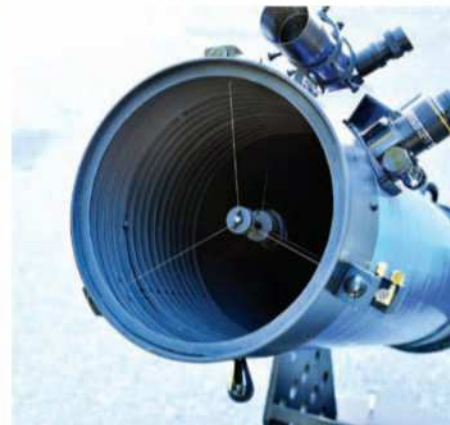
▲ Baffles at the front reduce stray light, while the wire secondary vanes minimise diffraction.
