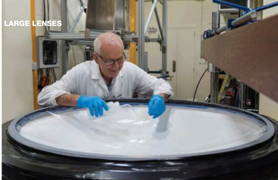
▲ LARGE LENS KiwiStar Optics' team leader of optical manufacturing, Dave Cochrane, cleans one of the six 1.1-metre lenses made for the William Herschel Telescope.
