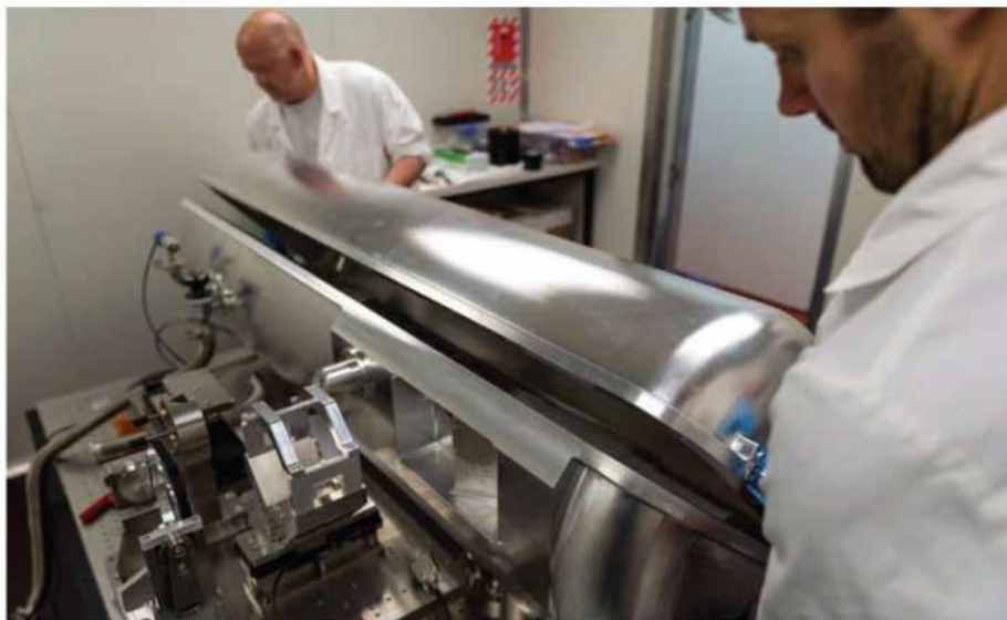
▲ LARGE LENS KiwiStar Optics' team leader of optical manufacturing, Dave Cochrane, cleans one of the six 1.1-metre lenses made for the William Herschel Telescope.
