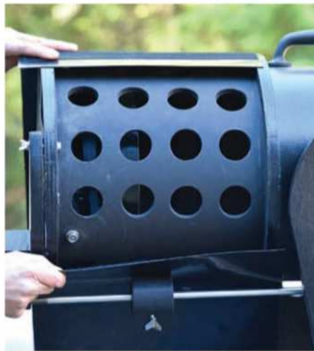
▲ Ventilation holes allow air to flow around the primary mirror, cooling it quickly. A shroud covers the holes to reduce stray light.
